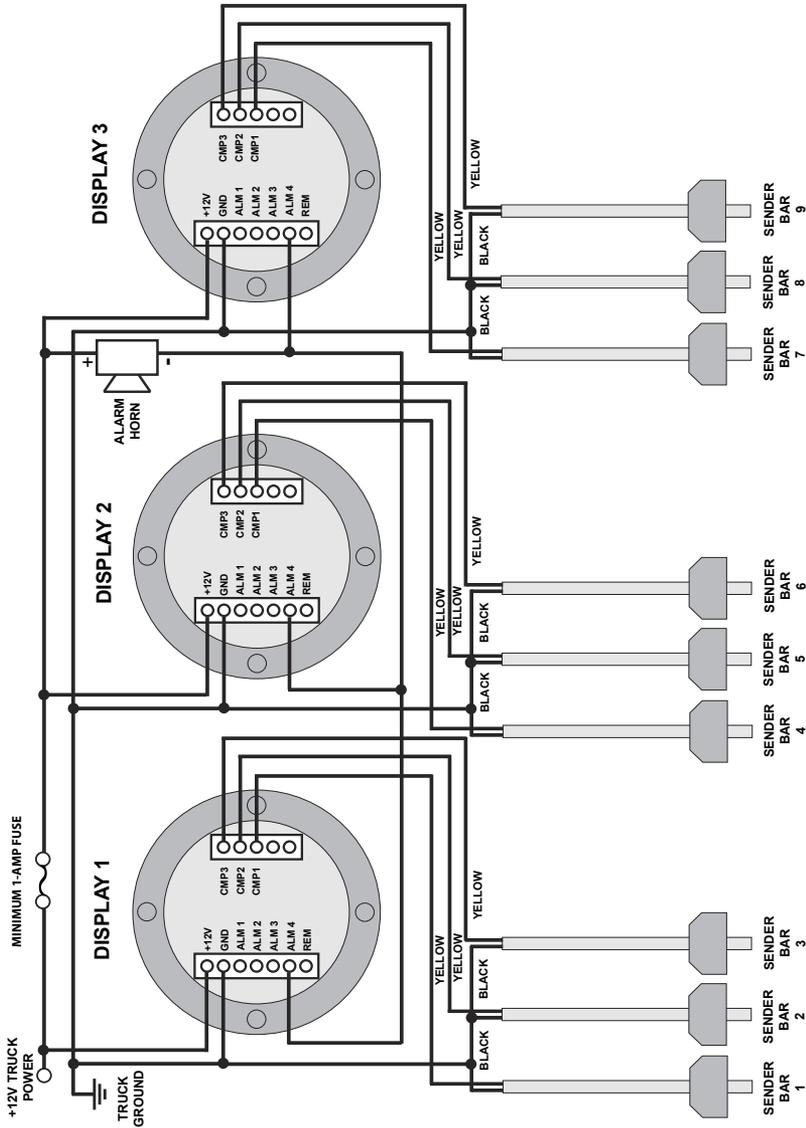
THIS EXAMPLE SHOWS 9 COMPARTMENTS CONNECTED TO 3 OUTSIDE DISPLAYS.
